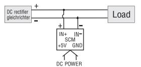
\* When serial SCM meters are installed, be sure to connect the power as one adopter (SP-0305) per one meter, because the meter is not insulated between input circuit and power circuit
